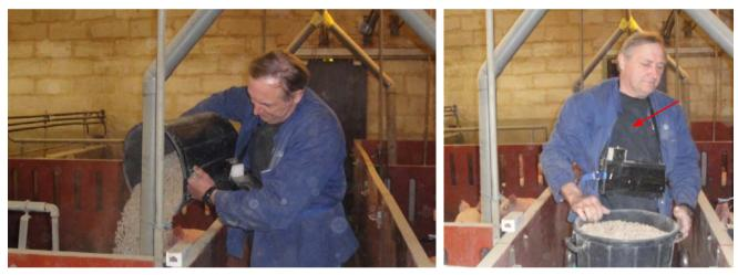
Figure 1. PM concentration measurements by personal sampling of the farmer during manual feeding. Sampling inlet is indicated with an arrow.
